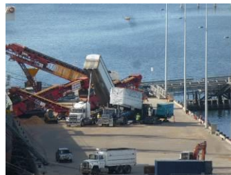
Trucks loading wood chips onto the conveyor – Rob Whiter
